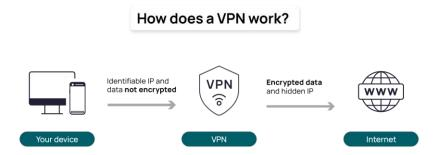
A VPN creates a secure, encrypted tunnel between a device and a remote network over the Internet.
